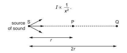
Air molecules at point P, a distance *r* from the source S, oscillate with amplitude  $8.0 \,\mu$ m.
